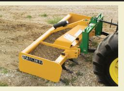
Box blades remove high points and fill in low points by scraping the surface and moving material across the work site. They're perfect for any job that requires precision scraping, leveling, and backfilling. Scarifier height is easily adjustable. Simply remove the shank key and raise or lower the scarifier to one of three settings. Use the low notch for deeper ground penetration.
