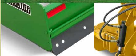
Tailgates are hinged to allow for clean material flow and improved leveling and finishing. Make the tailgate fixed simply by moving the locking bolts to the lower position. A fixed tailgate gives the cutting edge extra power to slice through hard, compacted ground. All 41 and 42 Series Hydraulic Box Blades come standard with a 2x4-inch hydraulic cylinder, pin kit and hydraulic hose kit.
