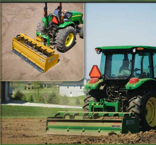
Cover more ground in less time with a low-back box blade, available in a variety of working widths. The low-back design (shown in green) reduces the weight of the implement, enabling you to carry a wider box blade behind your tractor. A high-back design (shown in construction yellow) also is available in select working widths.
