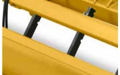
Scarifier height is easily adjustable. Simply remove the shank key and raise or lower the scarifier to one of four settings. Use the top notch for deeper ground penetration.
