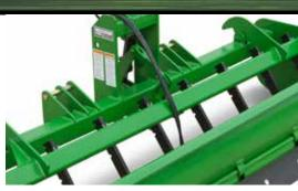
Knock out big jobs faster with the hydraulically controlled scarifier beam. You can raise the scarifiers up for backfilling and then lower them for scraping and leveling — all without leaving the tractor seat.
