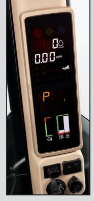
The cornerpost display is large and bright, making it easier to read fuel, temperature, engine speed, and ground speed.
