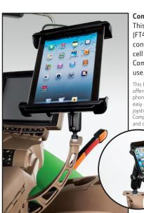
CommandARM™ bracket This bracket for Final Tier 4 (FT4) Tractors offers a convenient way to mount a cell phone or tablet to the CommandARM for easy
