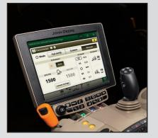
GreenStar™ 3 2630 Display comes ready with parallel tracking, field documentation, map-based prescriptions, harvest documentation and on-screen mapping. AutoTrac™and SectionControl can also be added to improve efficiencies even more.
