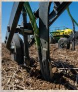
Feed the crop, not the weeds. Easily place fertilizer in dry, liquid or gas forms from 2 to 6 inches deep. Independent opener downforce can be set from 200 to 500 pounds with a trip clearance of 12 inches. The standard dry knife (shown)
