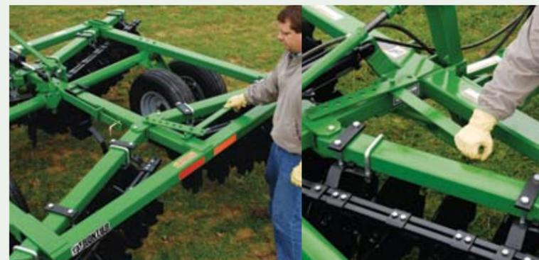
Gang angle adjustments are fast and easy. Just remove the locking pin and slide the gangs to one of nine settings.
