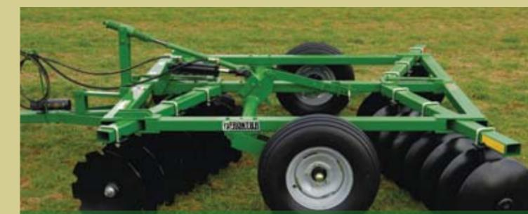
**Frontier DH1510 Disk** – for tractors with 45 to 75 horsepower – handles tough residue with ease. Its rugged construction and wider working width makes it ideal for moderate-sized fields. Choose from smooth or notched blades on 7.5-inch or 9-inch spacing. Working width is 10 feet 6 inches. (Shown with notched and smooth blades.)
