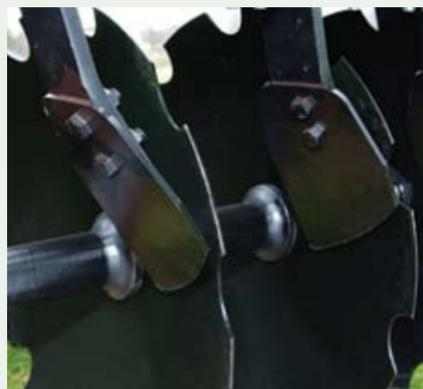
Adjustable blade scrapers are optional on all machines and keep you working in wet, sticky soil.
