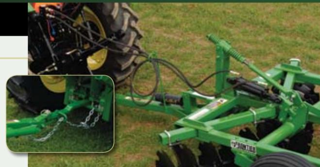
Hydraulic controls let you raise and lower the disk for transport without leaving the tractor seat. Safety chains are standard equipment on all models.
