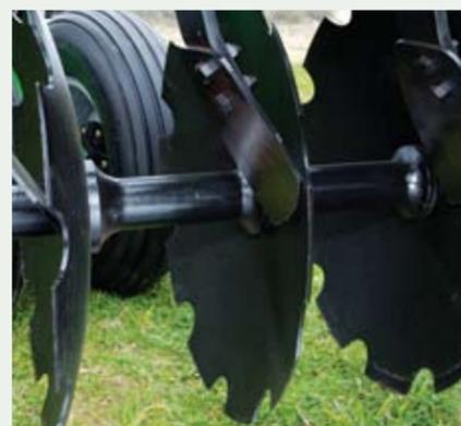
Choose notched or smooth blades with cast spools. Notched blades aggressively cut and mulch, while smooth blades slice and mix residue for a smoother finish. Also choose 7.5-inch or 9-inch spacing on both gangs, or 9-inch on front and 7.5-inch on back.
