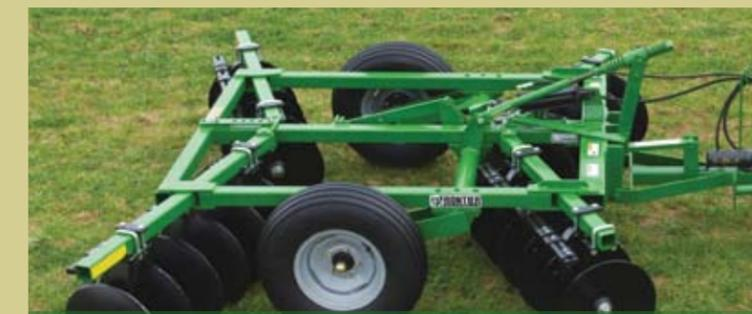
**Frontier DH1509 Disk** – for tractors with 40 to 65 horsepower – features the same rugged construction as the DH1508, but in a larger size. Choose from smooth or notched blades on 7.5-inch or 9-inch spacing. Working width is 9 feet 6 inches. (Shown with smooth blades and optional blade scrapers.)
