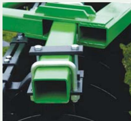
The rugged, heavy-duty tubular steel frame keeps the disk running smooth and level.
