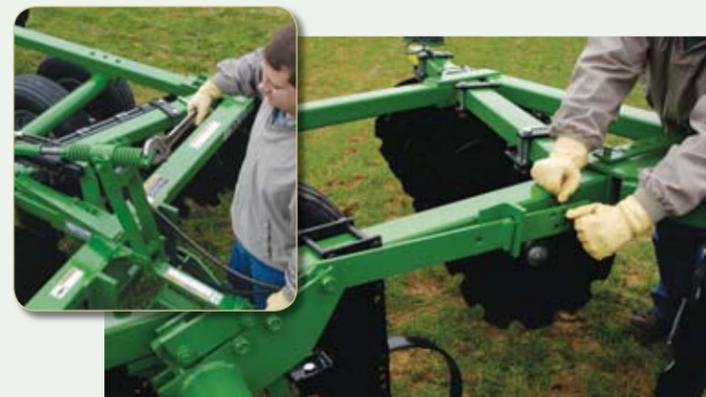
Crank-adjust front-to-rear leveling (left) lets you easily fine-tune disk leveling to avoid ridges and valleys in varying soil types and field conditions. Working depth is controlled with the depth-control bar (right). Simply position the pin and lock it into one of seven positions for the working depth you require.
