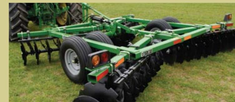
**Frontier DH1512 Disk** – for tractors with 55 to 80 horsepower – is the largest of the DH15 Series Disks. It's built to handle thick residue and tough field conditions. Choose from smooth or notched blades on 7.5-inch or 9-inch spacing. Working width is 12 feet. (Shown with notched blades, standard transport lights, optional furrow fillers, optional middle breaker, optional blade scrapers, and optional dual tires.)
