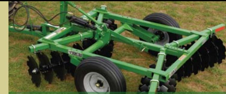
**Frontier DH1508 Disk** – for tractors with 35 to 55 horsepower – is built extra tough for a wide range of tillage chores ... from seedbed prep to incorporation. Choose from smooth or notched blades on 7.5-inch or 9-inch spacing. Working width is 8 feet. (Shown with notched blades.)
