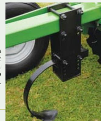
The middle breaker cuts out the center balk for a more level soil profile, ensuring complete coverage on each pass.
