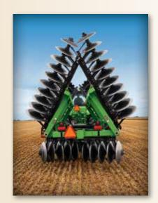
Disks are designed to provide maximum field coverage with each pass, yet convert to a narrow profile for easy transport. Dual folding cylinders allow both sides of the frame to hydraulically fold over to create a narrow transport width.
