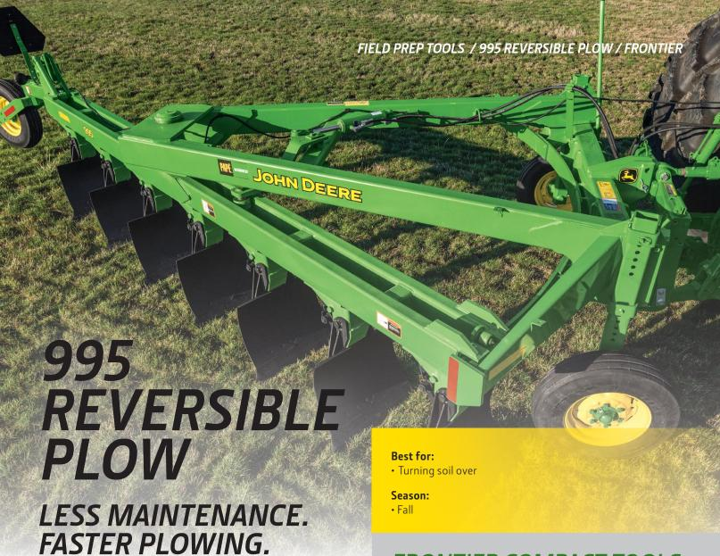
The John Deere 995 Reversible Plow pivot design lets you reverse the moldboards to make right- and left-hand-side passes to finish plowing faster. The on-land 995 Plow, available in 5, 6, or 7 bottoms, gives you maximum productivity from larger-horsepower tractors.
