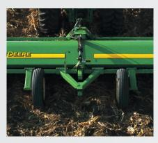
With this optional disk hitch, you can hook a disk behind the shredder to cut and till in one time-saving pass. A hydraulic hose support is also provided.
