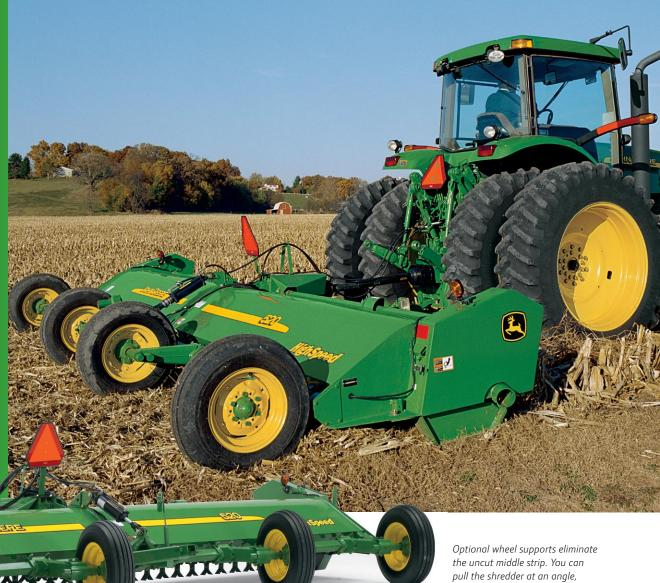
the uncut middle strip. You can pull the shredder at an angle, eliminating the middle strip.
