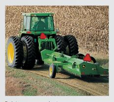
Endwise transport makes it easy to move your shredder. As an option on the 120, you can get permanent wheel arms for both operating and transport. Just remove one pin and move the wheels.
