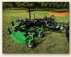
10 Series Flex-Wing Mower decks are made of 8-gauge reinforced steel and feature a round-tapered-style front deck for a closer trim.
