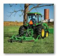
A round front, tapered rear deck design enables close mowing along trees, fences, building, and other obstacles.
