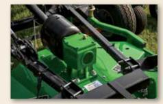
The rugged gearbox on the 10 Series Flex-Wing Grooming Mowers transfer power to the blades.
