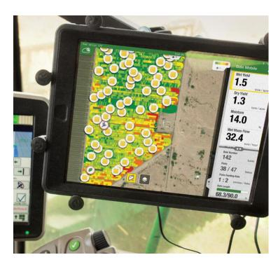
During and after baling, Bale Mobile allows you to track field performance, monitor bale quality and aid in retrieving bales.
