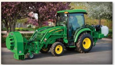
The BL2130 is shown above with the hydraulic power pack's optional oil cooler. Note to customers: The oil cooler option on the hydraulic power pack is recommended to regulate the hydraulic oil temperature.
