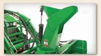
Control the direction of your discharge with quick and easy adjustments to the chute angle. Choose from standard manual chute deflection or optional hydraulic chute deflection (shown above).
