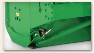
The SB2176 features adjustable skid shoes that minimize gouging on uneven surfaces, and provide added durability for longer wear life.
