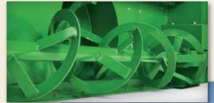
With a 64 or 76 inch (1.63 or 1.93 meter) working width and a sturdy 15 inch (38.1 cm) auger, you can move heavy volumes of snow with ease. Best of all, the Loader-Mount Snowblower monitors the amount of torque applied to the impeller allowing the auger to decrease speed when maximum torque is sensed, reducing the chances that the auger overloads the impeller. The result? Less chance for clogging the chute.
