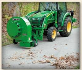
The BL2130 provides 141 mph (226.92 Km/h) maximum air velocity and 6,000 cfm (169.9 m³/min) maximum air flow for greater power when tough jobs approach.
