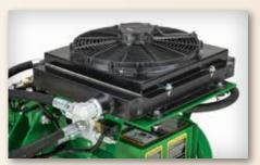
Optional oil cooler regulates temperature of the hydraulic oil when working in warmer environments.
