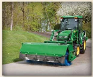
0 to 23 degree left or right angling allows you to windrow material without compromise. And optional gauge wheels let you set the height of the broom to match specific conditions.
