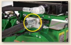
A standard internal thermal switch (highlighted) protects the hydraulic system from overheating, helping save on maintenance costs and minimizing downtime.
