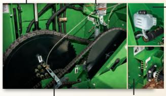
Drive system I The drive system features a heavy-duty clutch and chain for smooth power transfer and longer life. Shear bolt protection A rugged metal housing protects the shear bolt for longer life and uninterrupted performance. (Available only on MS2320 and MS2326 models.)
