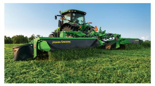
Paired with a tractor with a minimum of 210 horsepower, a front hitch and PTO, you can enjoy a comfortable cab environment while being able to change cutterbar angle without leaving the tractor seat. The convenience of quick-change knives allows you to change a knife in less than 15 seconds.
