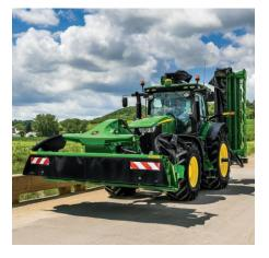
Not only can you cut wide, with up to a 32.5-foot (9.9m) cutting width, but you can transport narrow — at just over 11 feet. The rear-mount mowerconditioners fold up without leaving the cab, making transport fast and easy.
