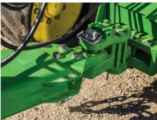
**The floating hitch and flexible frame** maintain consistent ground contact and uniform depth. The four-rank frame allows for high levels of residue to flow smoothly through staggered row-units, reducing downtime from plugging.
