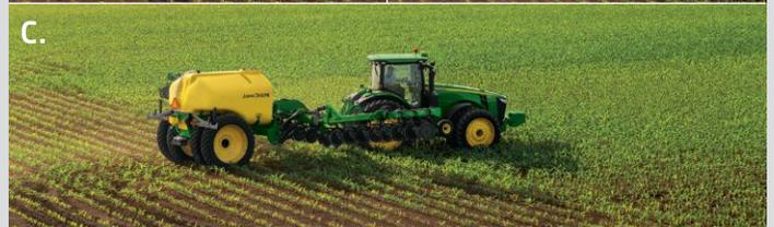
**Hydraulic wing kick** automatically lifts the wings higher than the main toolbar when turning in the field, providing increased clearance to greatly reduce any crop damage.
