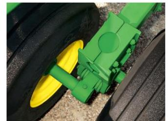
**The wheel and tire configuration** provide more flotation and even weight distribution across the entire machine.
