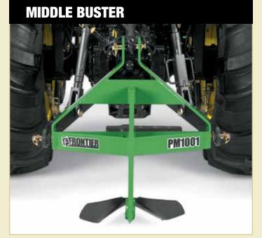
Use the Frontier Middle Buster to create planting beds for produce gardens. Equipped with a 19-inch double-wing cutting blade, the Frontier Middle Buster is perfect for planting vegetables and for digging up potatoes. Hook-up this gardening workhorse to your compact utility tractors with less than 45 HP.
