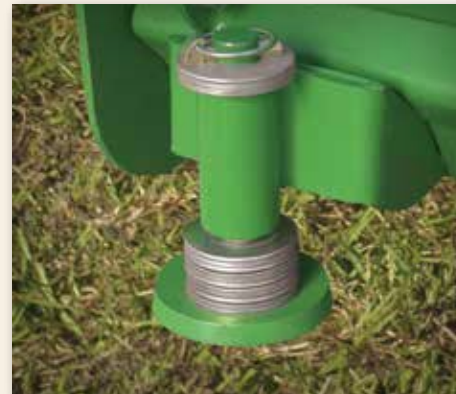
Optional skid shoes protect the moldboard cutting edge from hitting low-lying obstructions important when cleaning corrals or removing snow.
