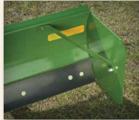
Optional end plates hold in extra material while pulling it from one place to another, making it an ideal feature for filling.
