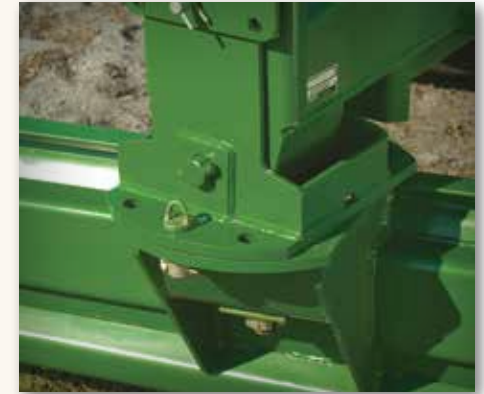
The turntable on the RB21 and RB22 Series allows you to adjust the angle to three different positions in both forward and reverse.
