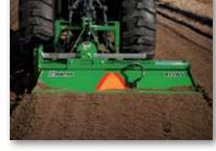
Adjustable offset allows the tiller to be used in a central or side position (pictured) with respect to the tractor's wheel track allowing you to till closer to existing plants and into deep corners. The chain-supported tailgate is self-leveling.
