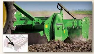
On the RT22 and RT23 Series, roller adjustment is easy using the two mechanical jacks placed on the sides of the rollers. Use a lower setting for more firming action, ideal for controlling wind erosion.
