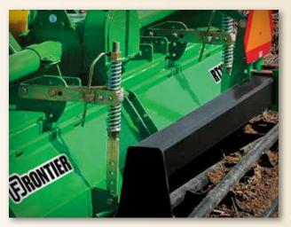
On the RT22 and RT23 Series, double springs provide consistent down pressure on the tailgate to level the tilled soil. Adjusting the height of the tailgate is easy: just remove the bolts and raise the tailgate to one of five settings. Use the low setting for a more level finish.
