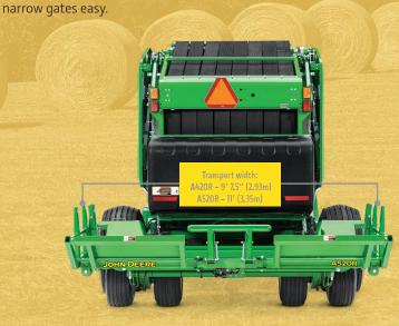
Our A520R Accumulator has the capacity to hold two 5 x 6' bales while making a third.
