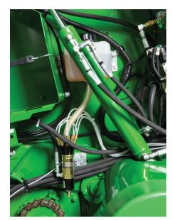
Lube Minder® Automatic Oiler Increase chain life with this fully adjustable chain oiler pump. Modify dispensing rates to ensure all chains and sprockets are properly oiled regardless of conditions. Specially engineered brushes clean chains and sprockets while applying oil to all moving parts while they're warm, allowing oil to penetrate pin and brush joints. Made in the U.S.A.
