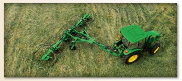
The TD3427 Hay Tedder is ideal for bigger fields. This rugged tool is offered in a 27-foot (8.23 m) tedding width and features six productive rotors – each with seven round tubular tine arms. Its hydraulic vertical fold with automatic tilt folds the tedder to 11-feet 6 inches (3.51 m) wide for easy transport. Hook this implement up to tractors with a minimum 55 PTO horsepower (41 kW).
