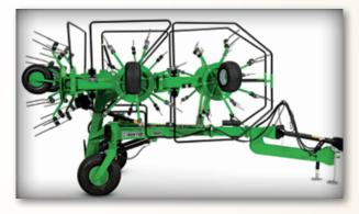
Each model features hydraulic folding for easy transport and storage. The TD3418 folds over center to 9-feet 2-inches (2.79 m), and the TD3427 has an integrated transport frame, allowing the implement to fold up and tilt forward to a compact 11-feet 6 inches (3.51 m) wide. For added convenience, the TD3427 has two independent transport wheels for greater ease and maneuverability. Transport lights are standard on the TD3427.
