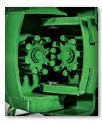
Both the TD3418 and TD3427 feature a finger joint drive system. The joints come together when the tedder is unfolded, providing smooth and reliable operation.
