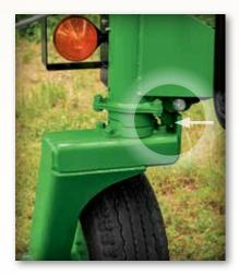
Locking cart wheels on the TD3427 keep wheels from swiveling during transport while allowing them to rotate freely in the field. The single-sided swivel design also helps prevent wrapping in long crops.
