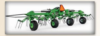
The TD3418 Hay Tedder is great for smaller operations, and is available in an 18-foot (5.49 m) tedding width. Seven round tubular tine arms extend from each of four heavy-duty rotor gearboxes. Designed for utility tractors with a minimum 30 PTO horsepower (22 kW).
