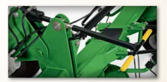
Tine height adjustments can be fine-tuned with the tine height adjustment lever. Simply turn the handle clockwise to raise the tines, or counter clockwise to lower the tine height. After tine height has been set, the hydraulic cylinder provides quick and easy raising and lowering of the tedder from the tractor seat.
